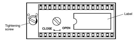
Mount the ROM to the socket in the direction indicated on the label and turn the tightening screw clockwise to the C (close) secure the ROM.
