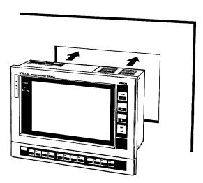
Use the accessory metal fittings and tool to fasten the PT to the panel surface. Do not use a screwdriver. A screwdriver may damage the fittings or the PT.
