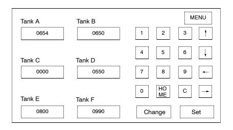
The screens used for these operations can be created in advance by using the "Support Tool" software on a personal computer. The screen data that is created using the Support Tool can be printed out, saved to a diskette, or transferred to the DT A TA CAMPACTATION, a Programmable Controller, or a compatible host.
