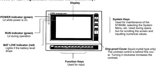
**Note** The operation of the BAT LOW LED will be unstable if a battery is not installed.
