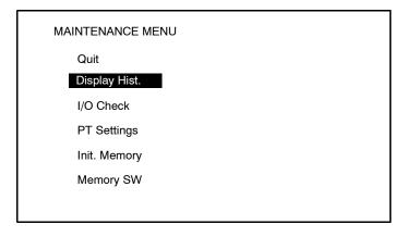
Move the bar cursor to History Record by pressing the Up and Down Keys. Then press the Enter Key.
