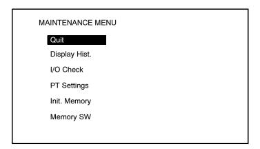
Move the bar cursor with the Up key and Down key, and select with the Enter Key.
