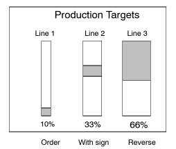
Note: When "with frame" is set for a graph, the width of the graph is reduced by two dots, so in that case the graph must have an original width of at least three dots.
