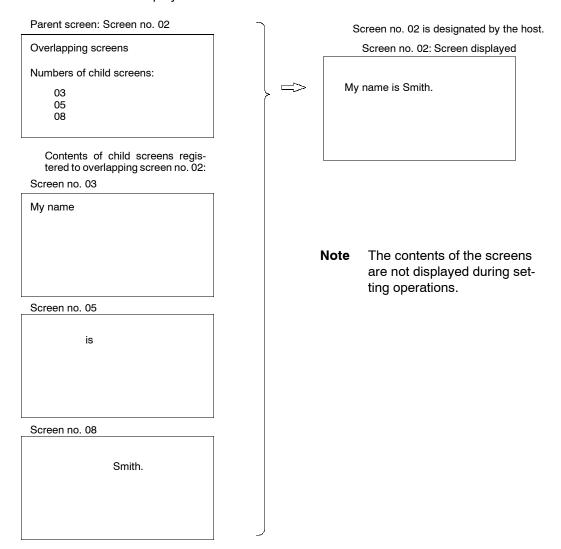
**Note** Parent screens (screen no. 02 in this case) cannot have screen data. They can be treated only as parent screens.
