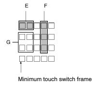
If switches E and F are turned ON simultaneously in this switch configuration, switch G will also turn ON.
