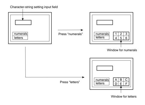
In order to make character-string settings, a key to confirm character-string input is required Allocate the Enter ( ) or ENT control key to a touch switch to
