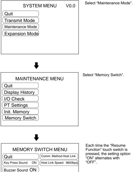
Each time the "Resume Function" touch switch is pressed, the setting option
