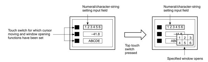
If the cursor moving keys are created automatically during creation of a numeral/ character-string input field with the support tool, the window opening function is not set. In this case, the window to be opened can be specified by modifying the touch switch.
