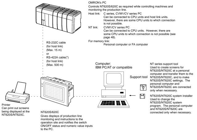
\* When the NT620S/NT620C is used with RS-422A, an RS-232C/RS-422 converter unit (NT-AL001) is required.
