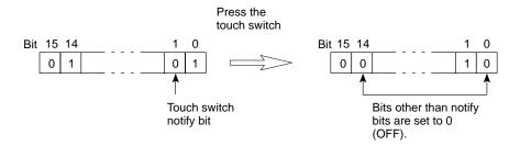
In the case of (2) in the table, since notification is executed on the basis of the contents of the word before display, the other bits in the word are not overwritten. However, if the contents of the word are changed at the PC during display, they will be rewritten based on the contents before display.
