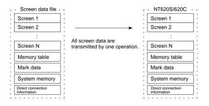
When screen data is transmitted from the support tool to the NT620S/620C, all existing screen data in the NT620S/NT620C is deleted.
