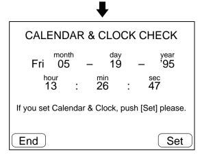
• After checking the date and time settings, press the "End" touch switch. The
