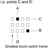
When switches A, B and C are switched on at the same time, switch D is also assumed to have been switched on due to the configuration of the touch switches.
