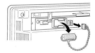
Install a new battery. Insert the battery connector, keeping it straight.
