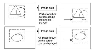
Image data of up to 224 images can be registered in a screen data file as code of FE20 to FEFF.
