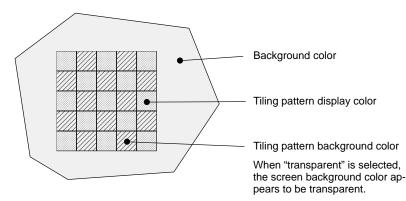
Part of the graphic frame may be invisible because of the combination of the display (in filling), background and outline colors. This phenomenon is peculiar to a color LCD, not a failure with the system.
