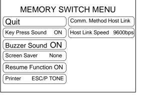
Each time the "Printer" touch switch is pressed, the next item in the applicable cycle of options below is selected:
