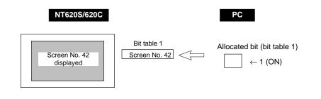
**Reference** The screens numbered 1997 to 1999 are earmarked for special functions, as shown below. The display history can be checked by calling them during operation.
