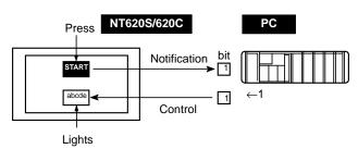
In order to notify the status of a touch switch to the PC, the touch switch must be allocated to a specified PC bit so that it can be managed. Designate the area and bit number.
