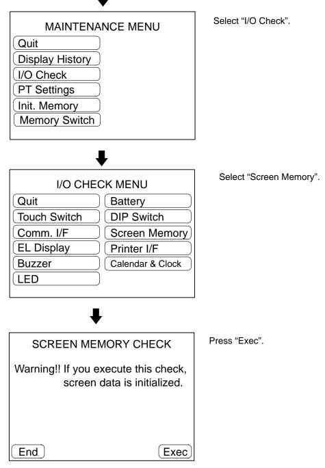
• If "End" is pressed without having pressed "Exec", the check is not executed.
