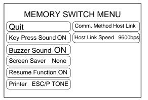
Each time the "Host Link Speed" touch switch is pressed, the setting option "9600 bps" alternates with "19200 bps".
