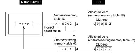
This specification method is a little complex, but it allows the display to be changed more easily according to the circumstances. In the example above, if 1 were added to the contents of memory table 18 to give 52, the contents of memory table 63 would be displayed instead.
