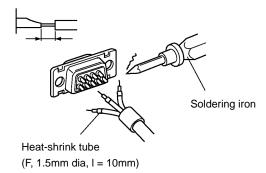
(4) Push the heat-shrink tube over the soldered joint and heat the tube to shrink it in place.
