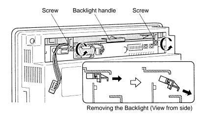
4. Insert the new backlight. Reversing the action in step 3, push the backlight in at an angle to start with, then, when it contacts something solid, continue by pushing it in straight. Now make sure that the positions of the screws that secure the backlight coincide with the positions of the screw holes in the top of the NT620C PCB.
