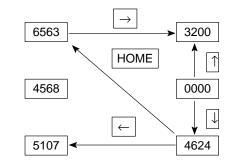
When the HOME key is pressed, the cursor can be moved at a stretch to an area at the upper left corner where a sum of XY coordinates is at a minimum
