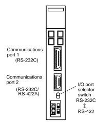
Two types of connectors are provided to CV500-LK201 host link unit. Both of these connector types can connect to the NT620S/620C with an RS-232C connector cable. Select the connector cable which matches the connector type.
