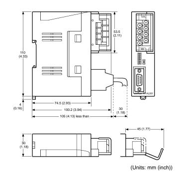
With RS-422A terminal block cover closed: 30 (W)  $\times$  114 (H)  $\times$  100.2 (D) mm
