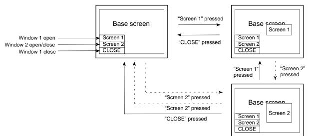
If an attempt is made to open a window that has not been registered, no window is opened (if a window is currently open, it will be closed).
