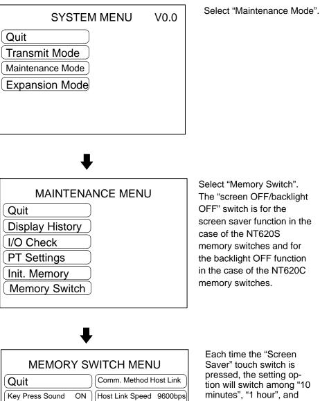
Each time the "Screen Saver" touch switch is pressed, the setting option will switch among "10 minutes", "1 hour", and "None".
