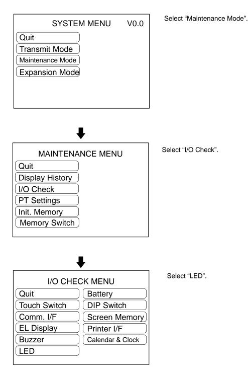
The "RUN" LED on the front face of the NT620S/620C will flash alternately green and red. The "POWER" LED will remain lit.
