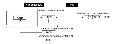
This method is convenient when switching the display at the same location, for example when monitoring a series of words, or when using unique codes to specify individual character strings, etc.
