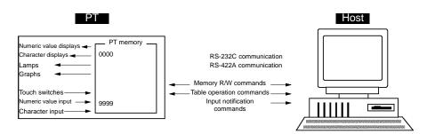
Therefore "memory link" is virtual direct connection executed at the NT620S/ NT620C and controlled by commands from the host.Memory link has the following restrictions when compared with host link and NT link.
