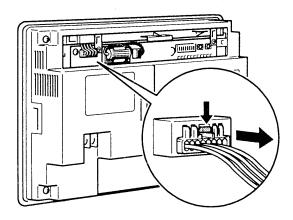
3. Remove the screws that secure the backlight with a Philips head screwdriver, grip the handle, and pull the backlight out (note that the screws are designed not to come out of the backlight). As shown in the figure below, the backlight can be removed easily if it is pulled straight out to begin with and then at a downward angle.
