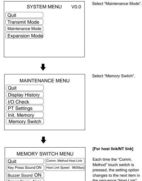
Screen Saver None Resume Function ON Printer ESC/P TONE pressed, the setting option changes to the next item in the sequence "Host Link", "NT Link", "1:N NT Link".
