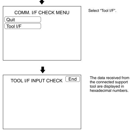
• When the check is finished, press the "End" touch switch. The "I/O CHECK MENU" will be redisplayed.
