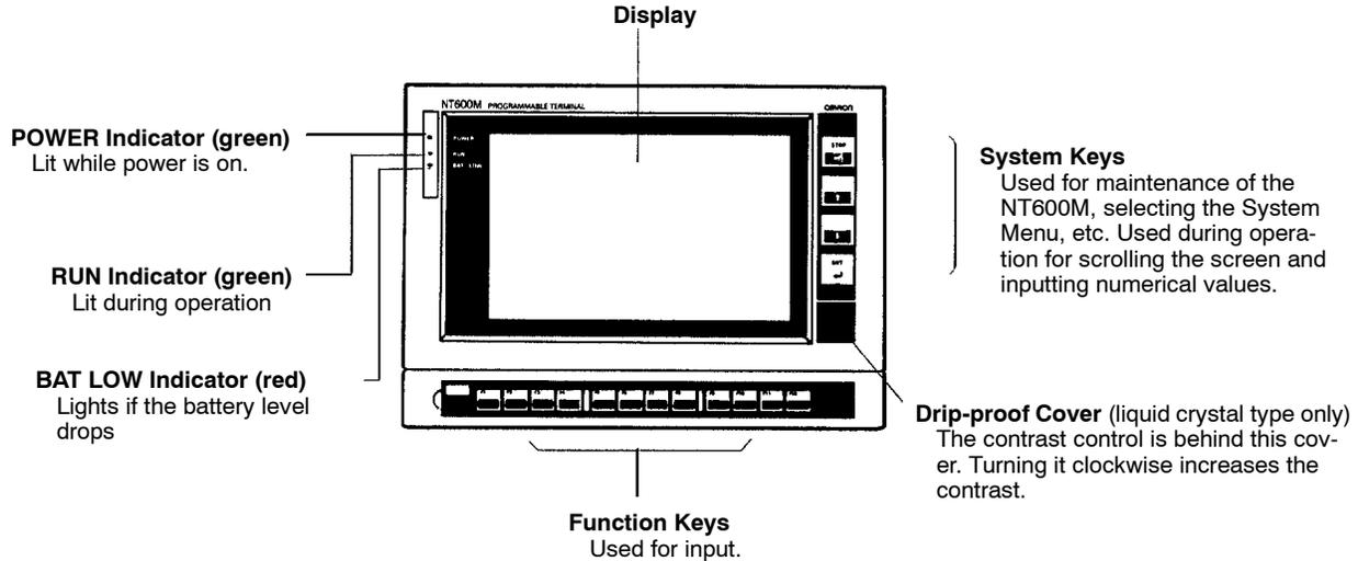
**Note** The operation of the BAT LOW LED will be unstable if a battery is not installed.
