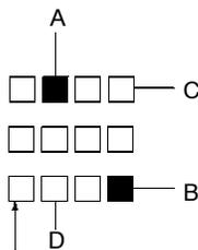
If switches A, B, and C are turned ON simultaneously in this switch configuration, switch D will also turn ON.
