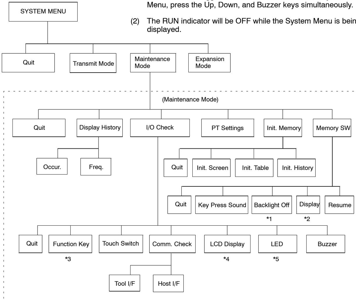
\*1: For PTs with EL displays, this becomes the residual image elimination function.
