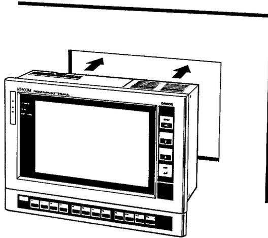
3. Use the accessory metal fittings and tool to fasten the PT to the panel surface. Do not use a screwdriver. A screwdriver may damage the fittings or the PT.
