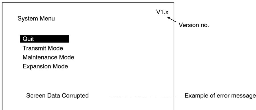
There are three types of error messages, as shown below. If an error message is displayed, first initialize the screen data memory before re-transmitting the data. Operation will not begin again until the error has been corrected.
