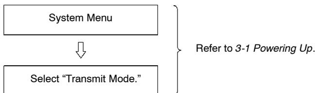
3. At the NT600M, it is only necessary to place the NT600M in Transmit Mode. The direction of transmission and the contents of the data to be transmitted are set at the Support Tool. (For instructions on operating the S... series Support Tool Operation Manual.
