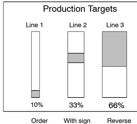
Note: When "with frame" is set for a graph, the width of the graph is reduced by two dots, so in that case the graph must have an original width of at least three dots.
