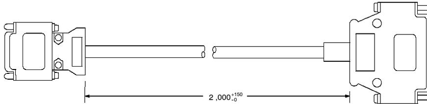
**Note** The personal computer end of the CV500-CN228 Connecting Cable is a 25-pin D-sub male connector. To connect to an IBM PC/AT or compatibles, a 9-pin or 25-pin D-sub female adapter is required.
