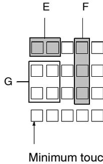
If switches E and F are turned ON simultaneously in this switch configuration, switch G will also turn ON.
