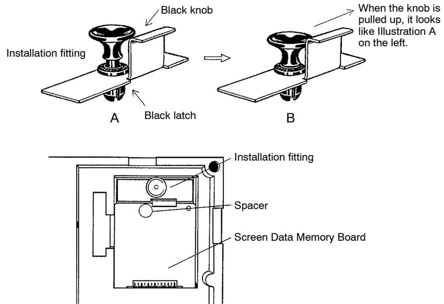
When removing the Screen Data Memory Board, first turn off the power to the PT and then remove the installation fitting by pulling up on the black knob. Then pull the Memory Board's spacer in the opposite direction of that shown above and take out the Memory Board.
