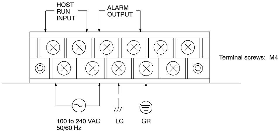
Use crimp-style terminals for wiring. If twisted wires are connected directly, there is a possibility of poor contact or short-circuiting. Use crimp-style terminals with holes to match M3.5 screws.
