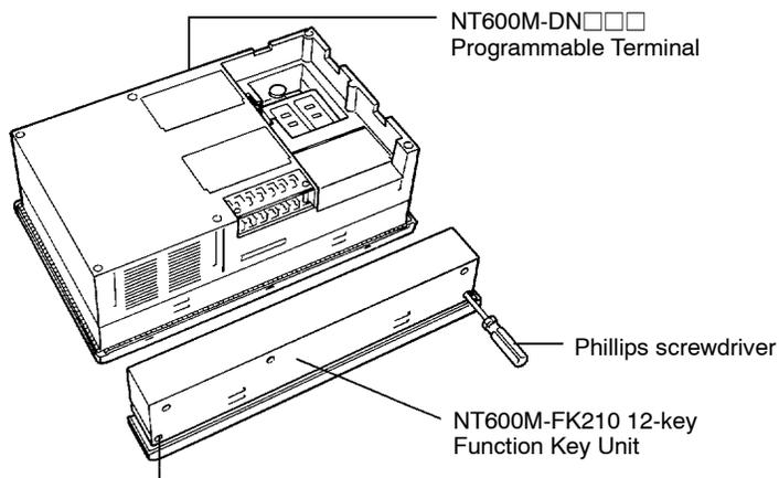
3. Attach the rubber packing that comes with the 12-key Function Key Unit.
