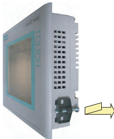
Example: Inserting plastic mounting clamps on the TP 177A
