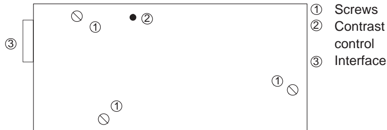
Figure 13-1 Rear of the OP3 Showing Screw Connections
