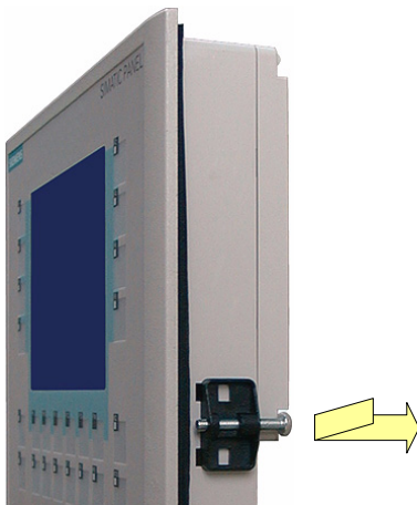
Figure 4-2 Inserting the spring terminals in the OP 170B
