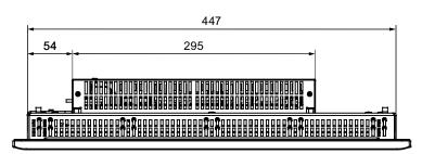
All dimensions in mm. Tolerance ±1 mm
