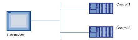
The operator can intervene in the operating process on the HMI device for control purposes. The controller in turn supplies the results of the operating process which are displayed on the HMI device.
