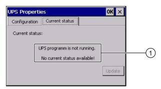
The "UPS program is not running. No current status available." message appears when the UPS is not connected.
