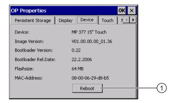
① Button for restarting the HMI device
