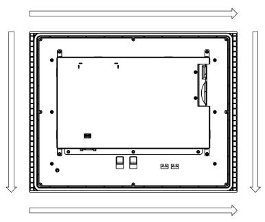
The following table shows the positioning of the mounting clamps on the MP 377 15" Touch. Observe the counting direction.
