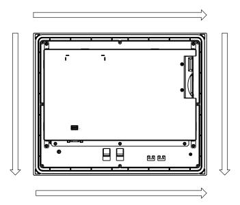
The following table shows the positioning of the mounting clamps on the MP 377 12" Touch. Observe the counting direction.
