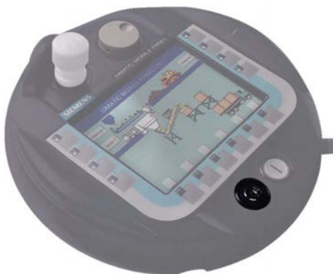
Picture 6-15 Key-operated switch
