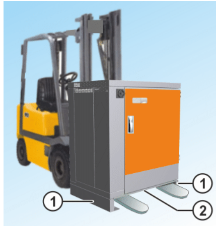
Fig. 7-2: Transportation with standard cabinet base
