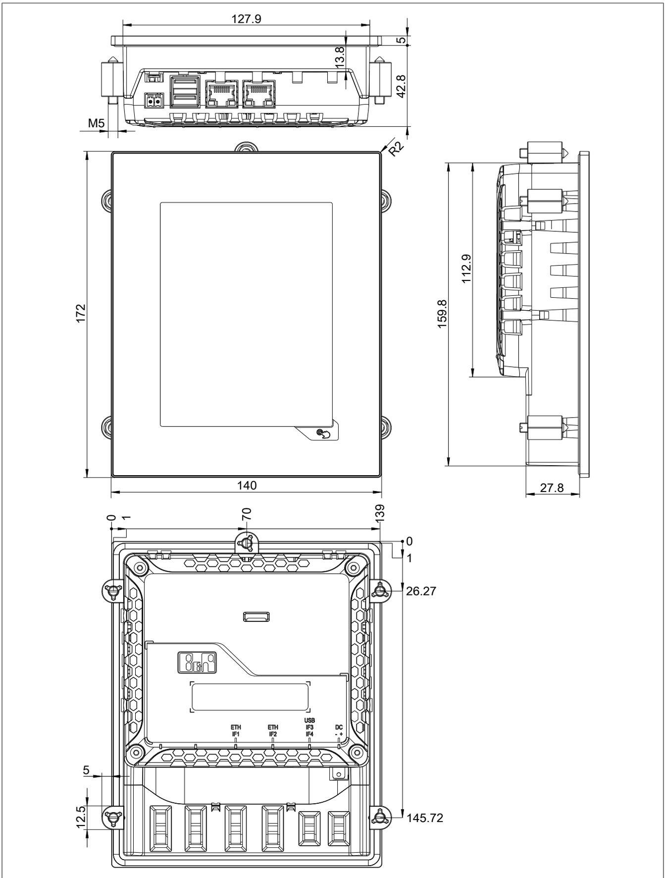
Figure 15: 6PPT30.057x-20x - 6PPT30.057L - Dimensions
