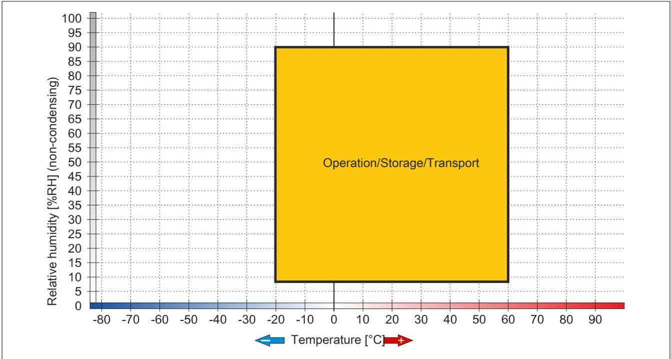
Figure 5: 6PPT30.043x-20x - Temperature/Humidity diagram
