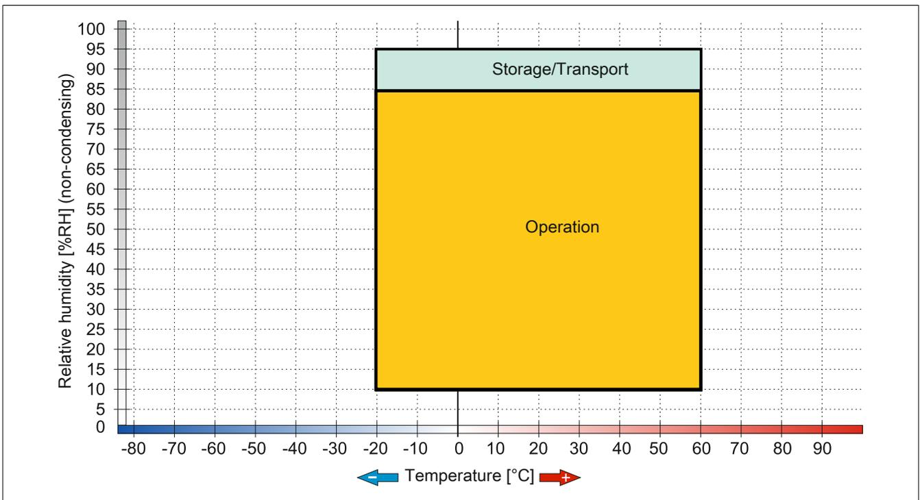
Figure 8: 6PPT30.101x-20x - Temperature/Humidity diagram
