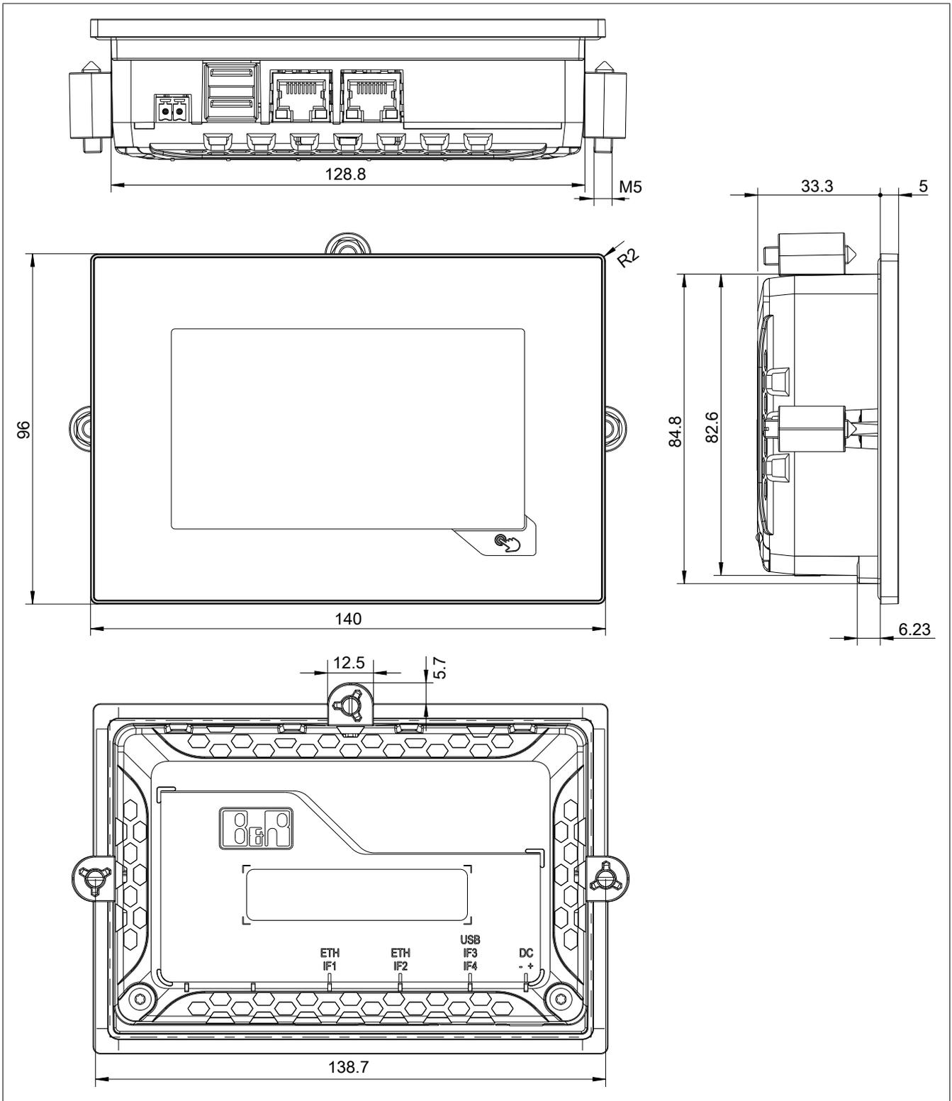
Figure 12: 6PPT30.043x-20x - 6PPT30.043F - Dimensions
