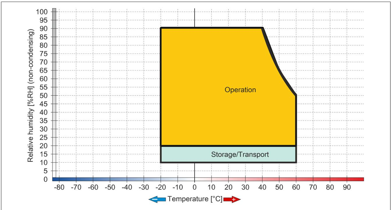
Figure 7: 6PPT30.070x-20x - Temperature/Humidity diagram
