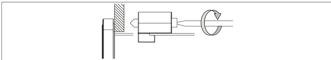
Figure 23: Mounting with retaining clamps
