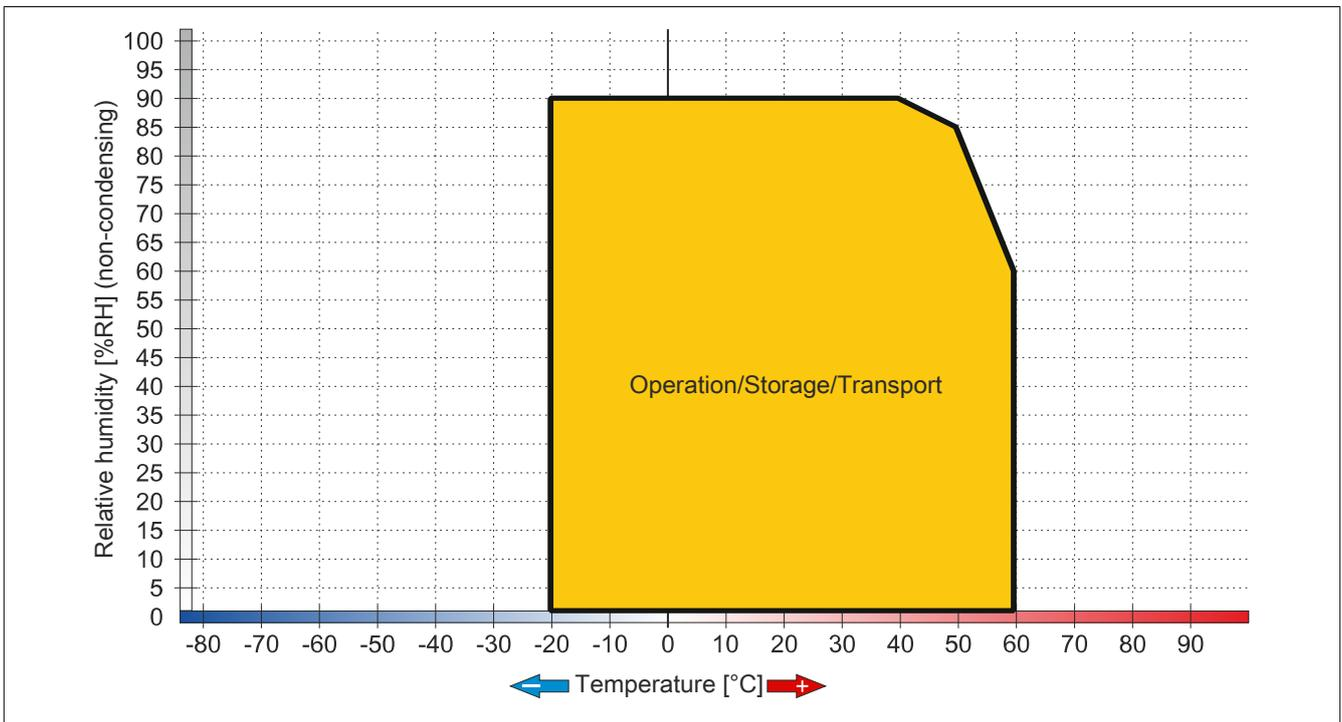
Figure 6: 6PPT30.057x-20x - Temperature/Humidity diagram
