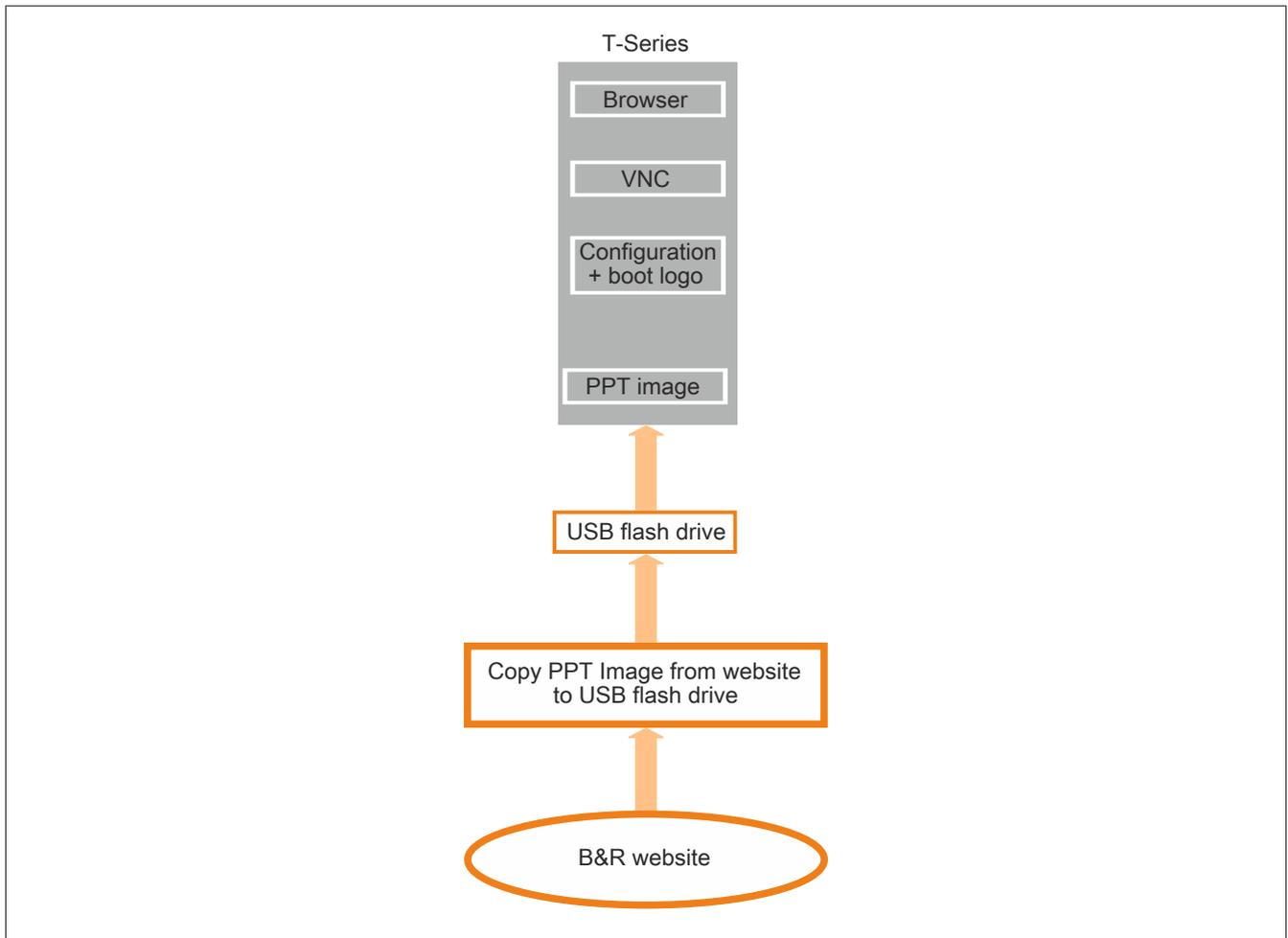
USB flash drive data is generated for the PPT image update via download from the B&R website. The Power Panel is then updated by connecting the USB flash drive.
