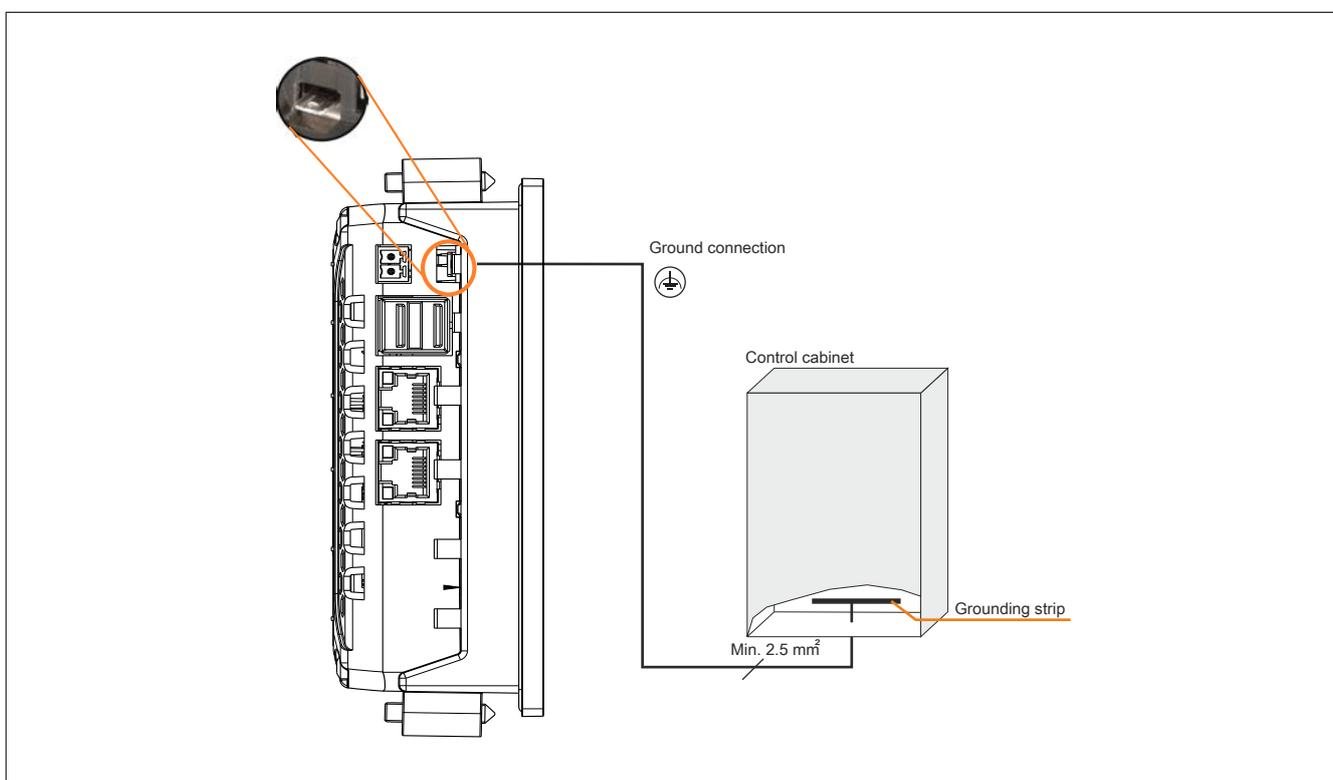
Figure 27: Power Panel - Ground connection
