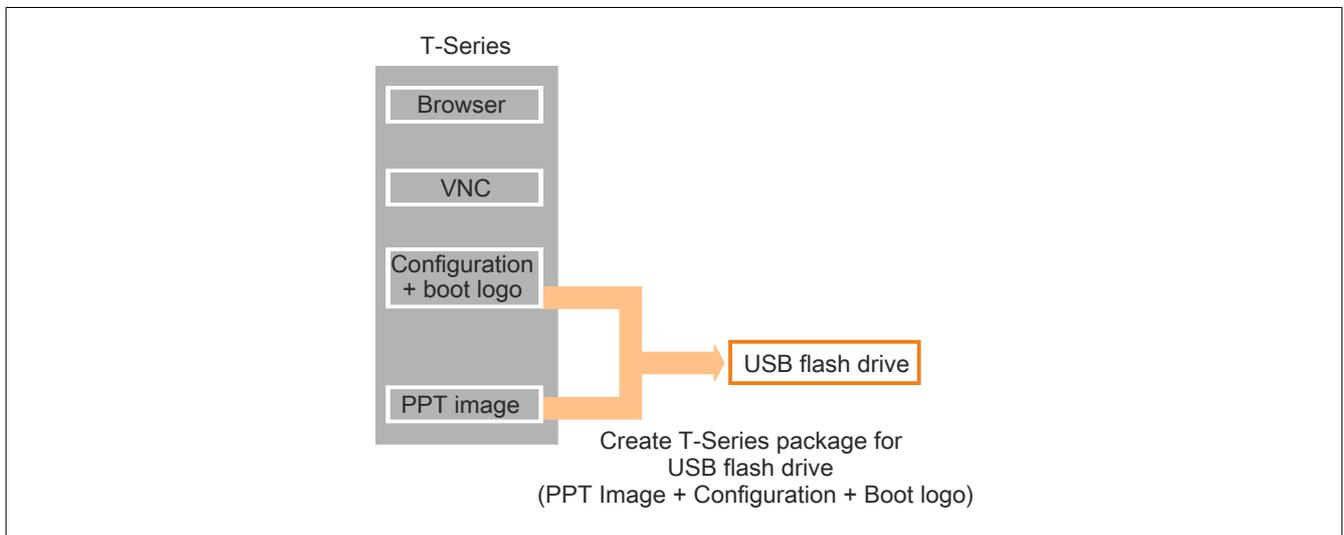
The USB flash drive data is generated for the PPT image and configuration and boot logo update for completely assembled Power Panels (via the configuration page). All additional Power Panels are then updated by connecting the USB flash drive.
