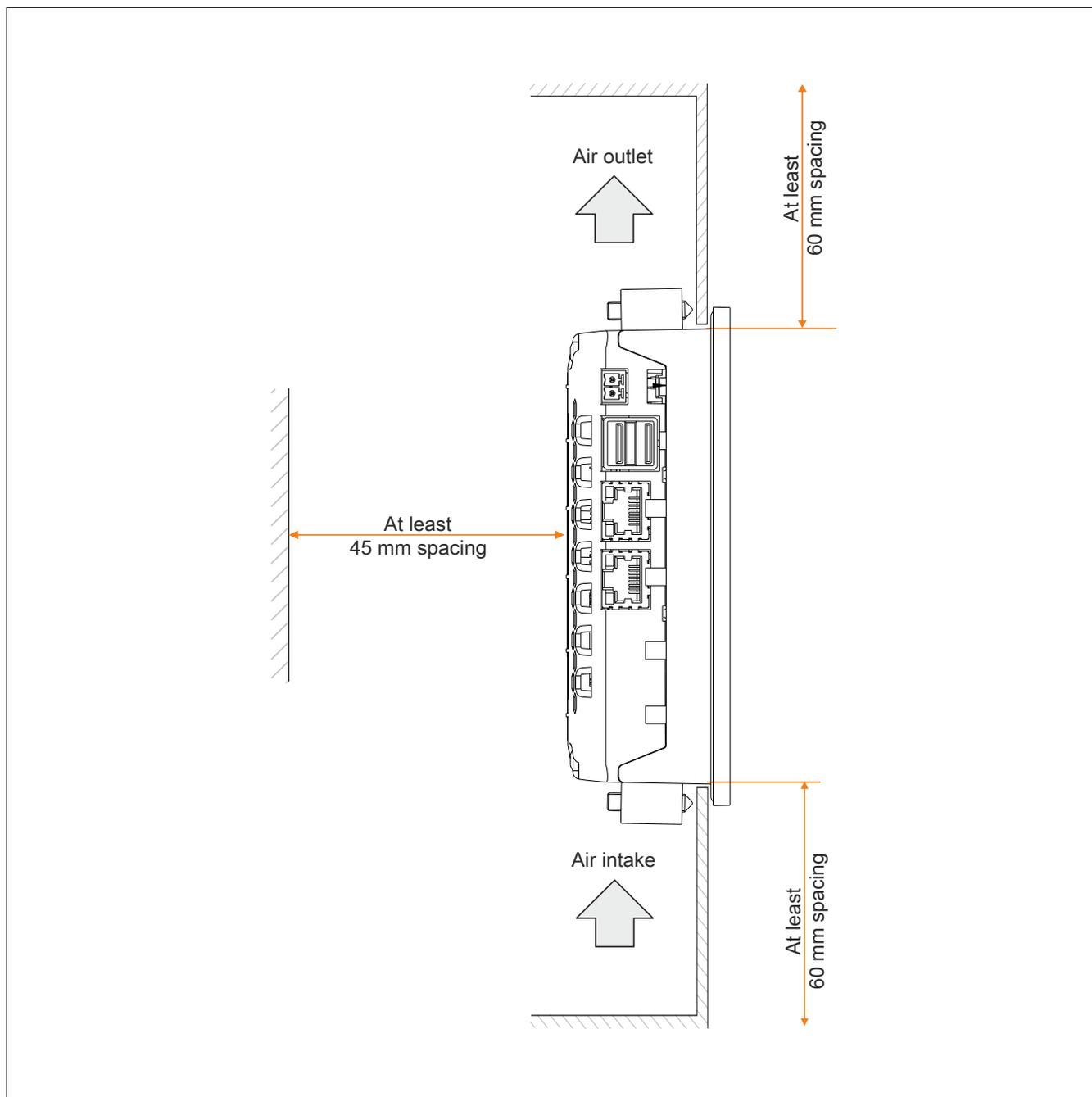
Figure 25: Spacing for air circulation - Side view
