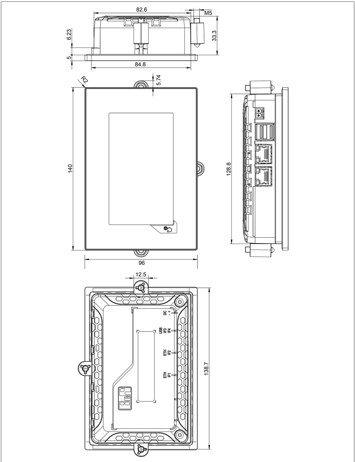
Figure 13: 6PPT30.043x-20x - 6PPT30.043K - Dimensions
