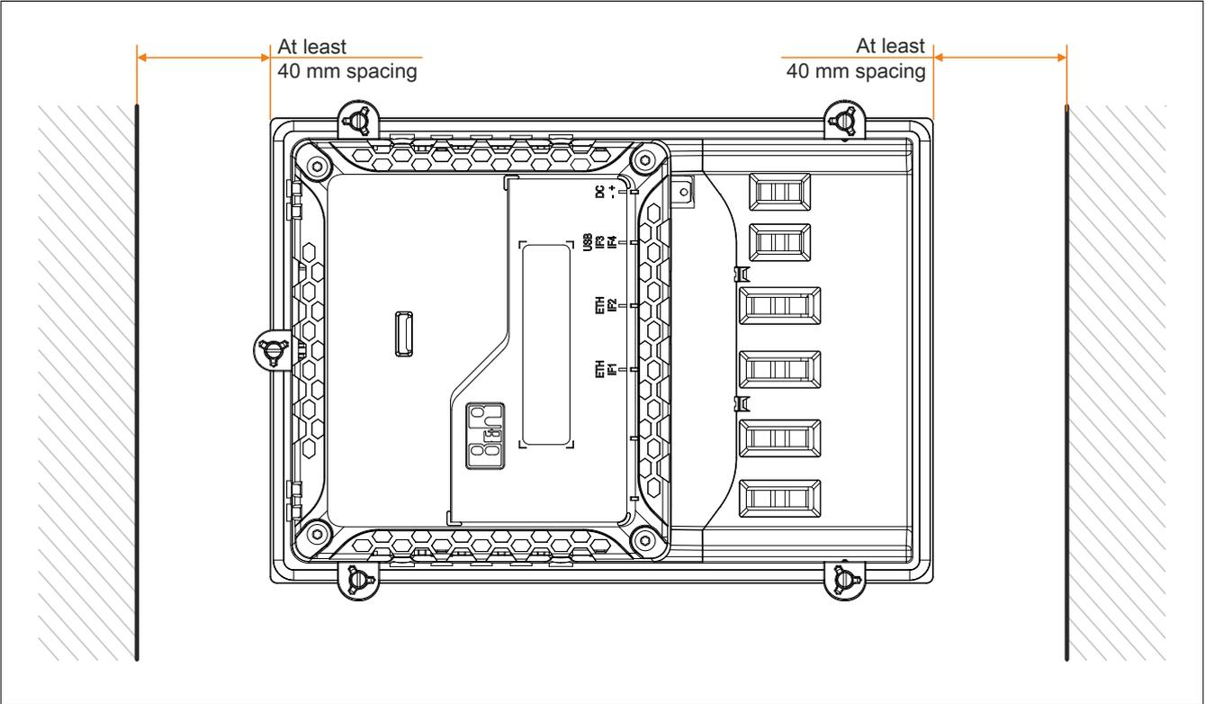
Figure 24: Spacing for air circulation - Rear view
