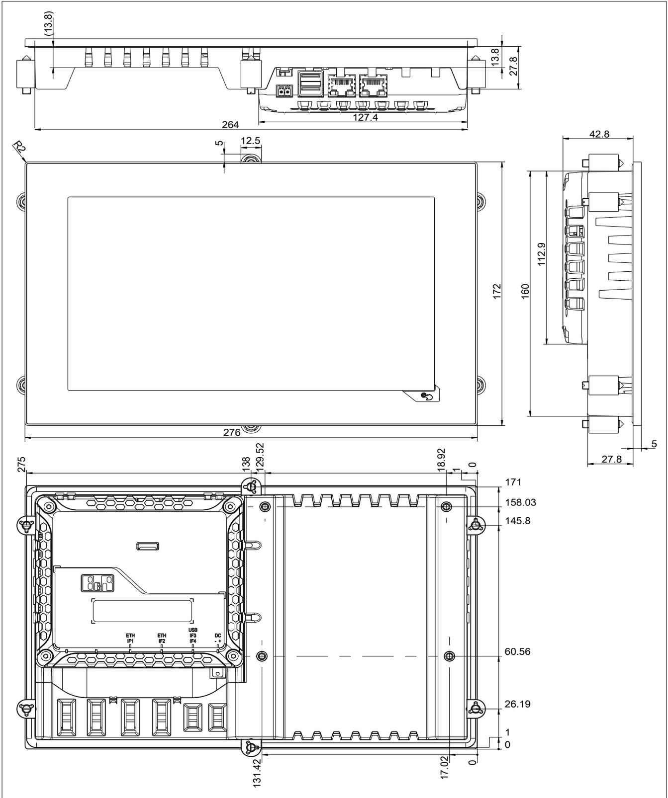
Figure 18: 6PPT30.101x-20x - 6PPT30.101G - Dimensions
