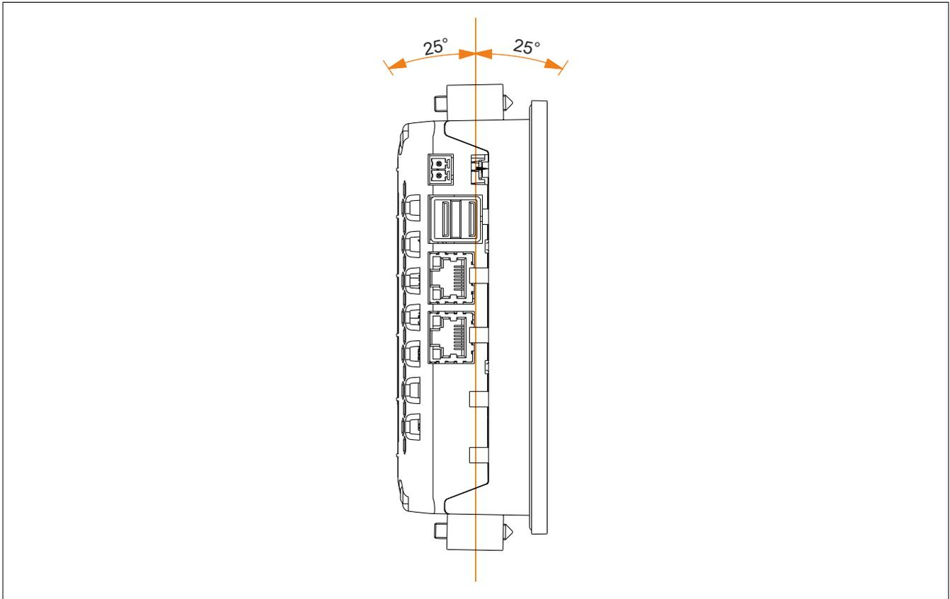
Figure 26: Power Panel - Mounting orientations
