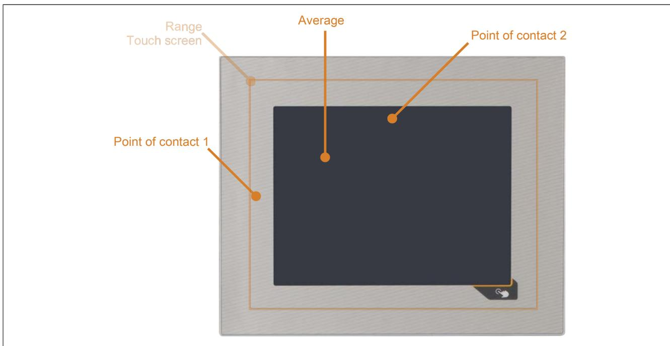
Figure 29: The midpoint between 2 points of contact
