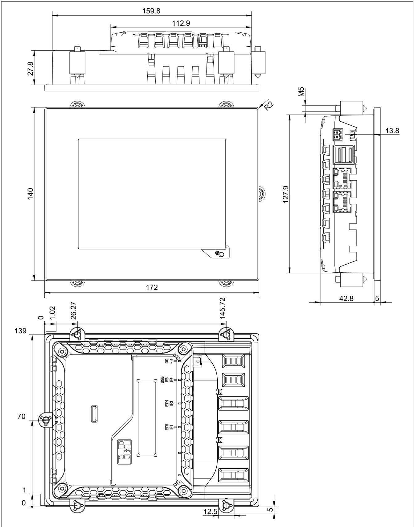
Figure 14: 6PPT30.057x-20x - 6PPT30.0573 - Dimensions
