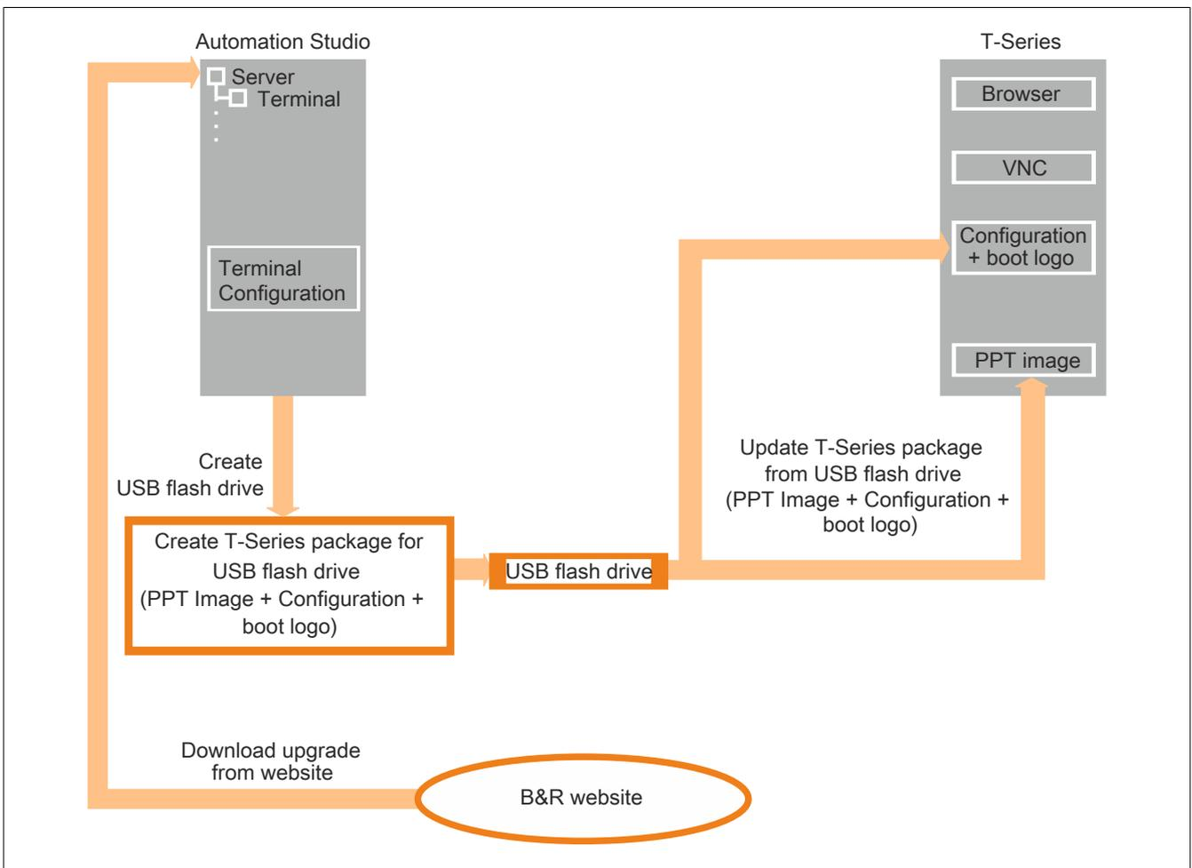
The USB flash drive data is generated for the PPT image and configuration as well as the boot logo update in AS. The Power Panel is then updated by connecting the USB flash drive.
