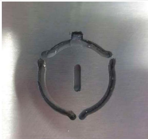
Figure 82: Cut the panel overlay along the cutout areas
