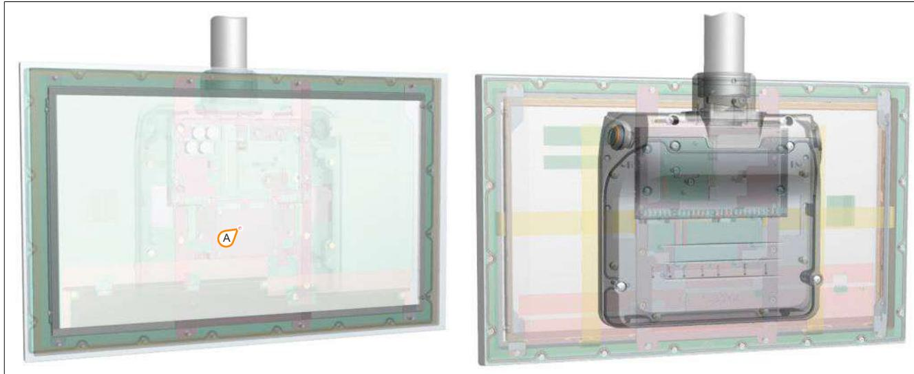
Figure 11: Automation Panel 5000 - Temperature sensor position
