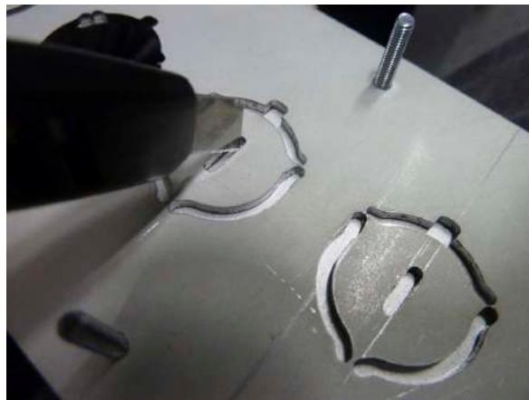
Figure 83: Cutting two parallel slits
