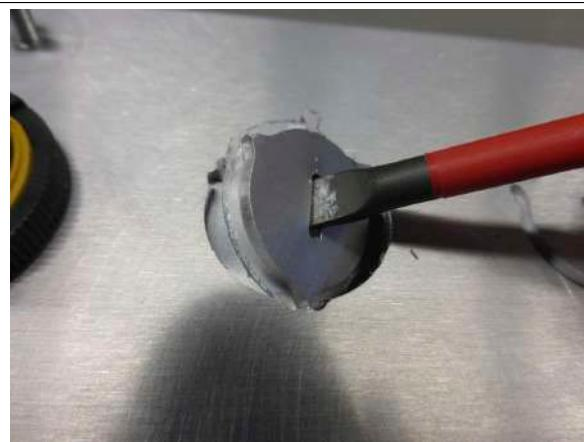
Figure 84: Breaking through the cutout for the operating element from the inside
