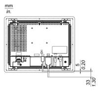
**NOTE:** All the above values are designed with cable bending in mind. The dimensions given here are representative values depending on the type of connection cable in use. Therefore, these values are intended for reference only.
