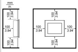
The holes on the rear of the panel (except HMIGTO1300/1310) do not correspond to VESA 75 mm standards. Do not attach the panel to a commercial-type VESA arm.
