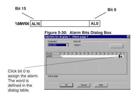
Click **Add** to assign the alarm bit (bit 0 of word %MW104) (Figure 5-30).
