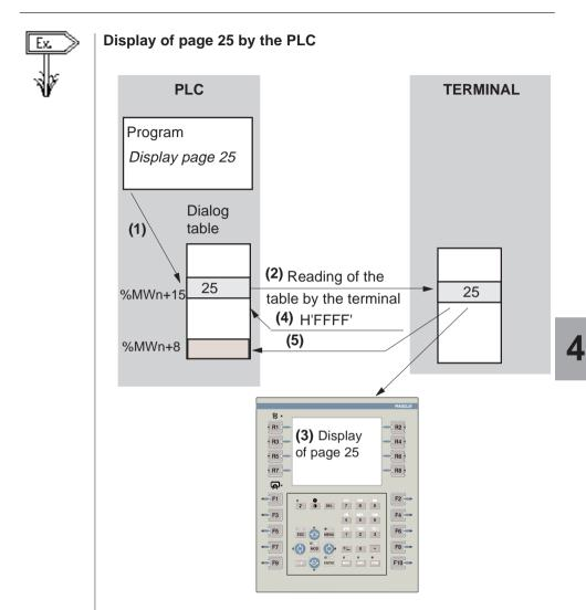
(1) The PLC writes in the dialog table the number of the page to display, 25. (2) The terminal periodically reads the dialog table in the PLC and (3) displays the required page. Once the command has been processed, (4) the terminal writes H'FFFF' in the word "Number of the page to be processed" and (5) the number of the displayed page in the word "Number of the displayed page."
