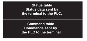
The number of words in the table depends on the choice of status data and commands that are to be processed during the dialog. The XBT-L1000 software allows you to configure the dialog table (Figure 4-1).
