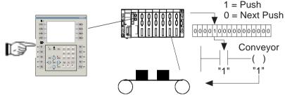
The XBT-L1000 software allows you to assign the desired command to each function key.
