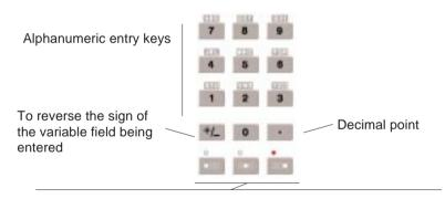
Combined with the alphanumeric keys, these keys give access to the character situated on the left, in the middle, on the right of the group of letters. The indicator lights indicate if letter entry is possible.
