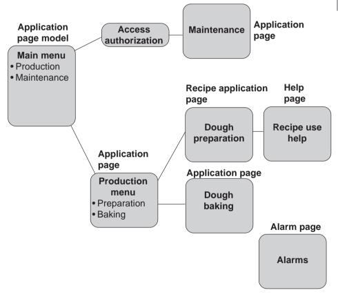
An **application page Model** will be used to display the company name and logo on the application pages (Dough preparation, Dough baking, Maintenance).
