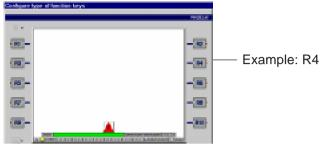
2. Select Action/Page access, the destination page (Dough preparation), click Image and insert the image associated with the R4 key (see Section 5.3.2 importing an image) (Figure 5-17).
