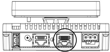
Do not confuse the RJ45 Ethernet connector with the RJ45 COM1/COM2 serial port.
