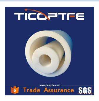
PTFE moulded tube can be made into non-standard parts by mechanical working, also it can be used as non-sticking materials. It can be used at the temperature of  $-180^{\circ}\text{C} \sim +260^{\circ}\text{C}$ . It has the lowest frictional factor and the best anti-corrosive property among the known plastic materials.
