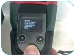
"M" Function Key: Preset, Maint. Count, Life Count, Information, Password, Back.
