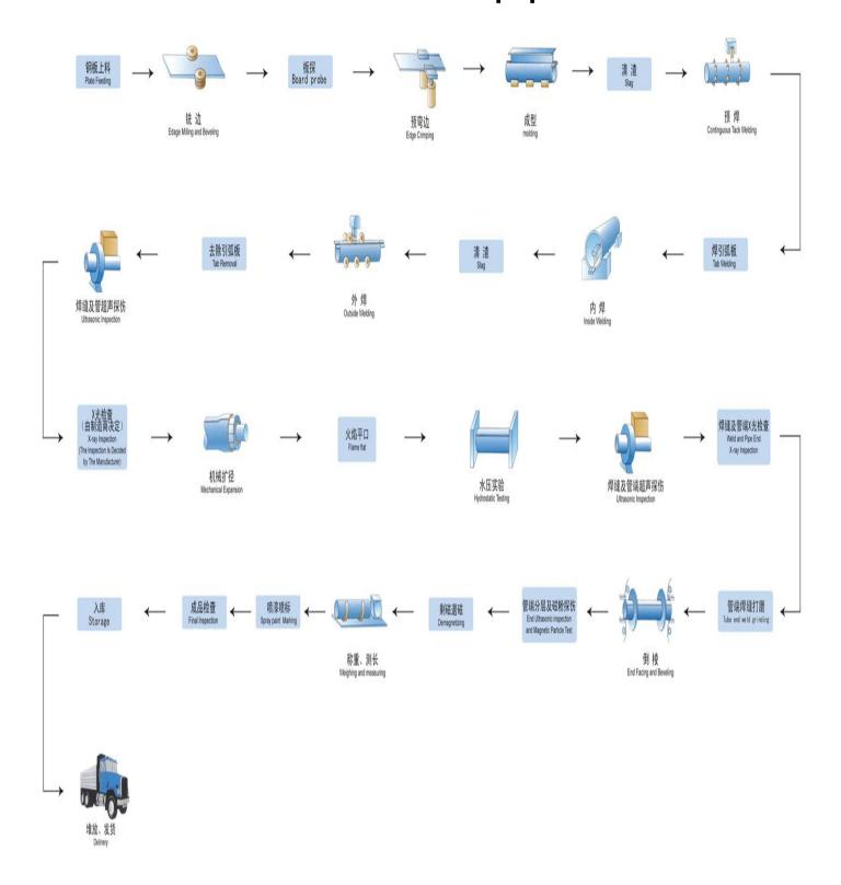
Plate Edge Milling Machine, Plate Edge Crimping Machine, Forming Machine, Tack Welding Machine, and the Mechanical Expansion Machine, producing by the professional manufacturer of large diameter submerged arc welding equipment, are all adopt the first-class design and manufacture technology internationally, with the PID control automation and online nondestructive testing automation control, it is prestigious in the field of Steel pipe equipment manufacturing
