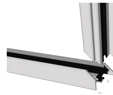
被动扇上口按图切角 Passive sash upper opening chamfer according to the diagram
