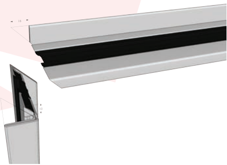
被动扇按图切角 (两端对称) Passive sash chamfer according to the diagram (symmetrical at both ends)
