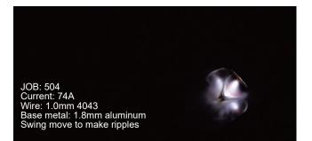
With the advanced Pulse MIG, you can easily get a cosmetically pleasing weld seam, with significantly lower and more controller heat input into the workpiece. It results in much lower distortion and less rework, very suitable for welding the thin Aluminum sheets.
