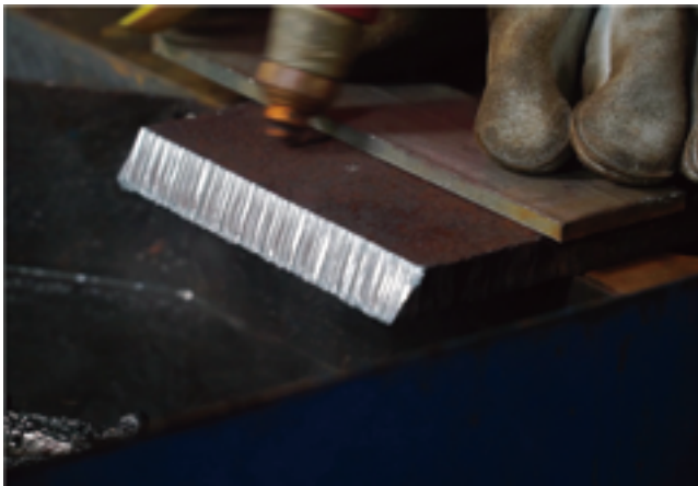
*16mm M.S. 60° bevel cutting by PROCUT-75MAX
