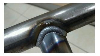
Thin (less than 2mm) pipes or frame/structure welding jobs, like the furnitures etc.
