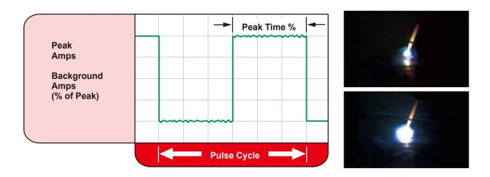
Typically from 0.2 to 10 PPS. Provides a heating and cooling effect on the weld puddle and can reduce distortion by lowering the average amperage. This heating and cooling effect also produces a distinct ripple pattern in the weld bead. The relationship between pulse frequency and travel speed determines the distance between the ripples. Slow pulsing can also be coordinated with filler metal addition and can increase overall control of the weld puddle.
