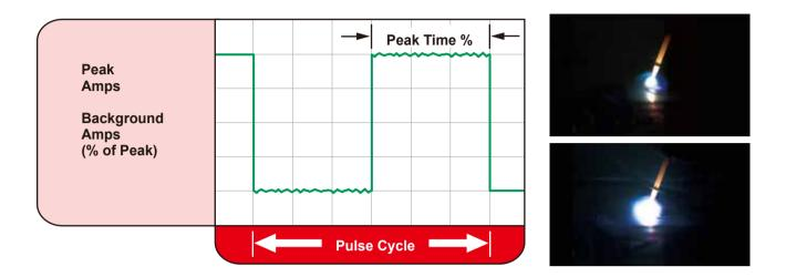
Typically from 0.2 to 10 PPS. Provides a heating and cooling effect on the weld puddle and can reduce distortion by lowering the average amperage. This heating and cooling effect also produces a distinct ripple pattern in the weld bead. The relationship between pulse frequency and travel speed determines the distance between the ripples. Slow pulsing can also be coordinated with filler metal addition and can increase overall control of the weld puddle.
