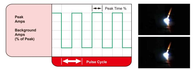
In excess of 40 PPS, Pulsed TIG becomes more audible than visible—causing increased puddle agitation for a better as-welded microstructure. Pulsing the weld current at high speeds — between a high Peak and a low Background amperage — can also constrict and focus the arc. This results in maximum arc stability, increased penetration and increased travel speeds.
