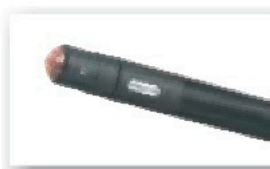
PLASMA torch: Trafimet A 141P Voltage class: M Standard Length: 6M Air consumption: 210 l/min Air pressure: 5 bar Duty Cycle 60%: 140A Duty Cycle 100%: 100A Ignition: HF
