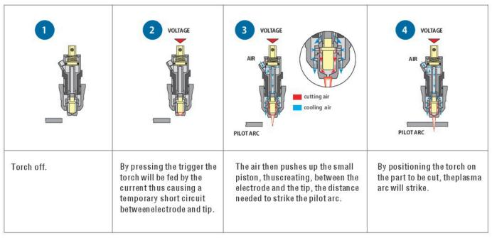
Less electromagnetic disturbance, with consequent absence of problems for any electronic, radio, television, telephone and computer systems in the vicinity of the cutting positions.
