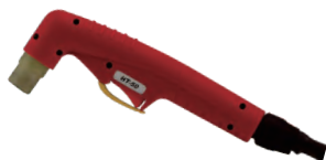
Plasma torch: HT-50CB Current: 50 Amp Duty Cycle: 60% Gas: AIR Gas Pressure: 4.5-5.0 Bar Gas Flow: 120 LPM Ignition: HF Post Flow: 50 sec.recommended Standard Length: 6M
