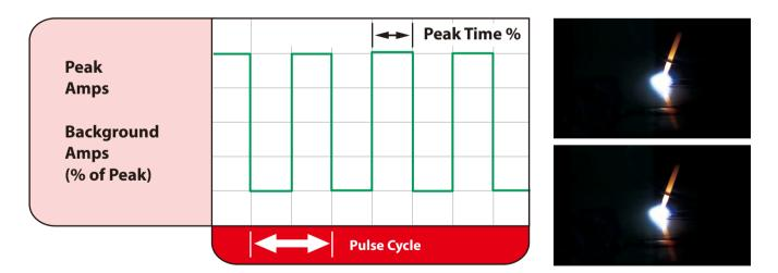
In excess of 40 PPS, Pulsed TIG becomes more audible than visible—causing increased puddle agitation for a better as-welded microstructure. Pulsing the weld current at high speeds — between a high Peak and a low Background amperage — can also constrict and focus the arc. This results in maximum arc stability, increased penetration and increased travel speeds.
