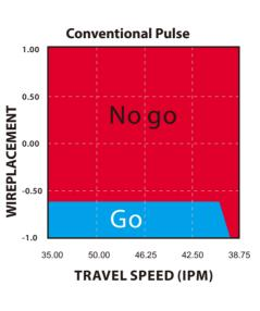
The green area represents wire placement and travel speeds at which acceptable welds are made. The red area represents unacceptable welds.
