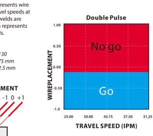
Pulse-On-Pulse made good welds at faster travel speeds over a wider range of wire placement.
