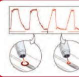
The high energy pulses provide a hotter arc (longer arc duration), which improves cleaning action at the base material. The low energy pulses allow the weld puddle to cool, which controls the heat input for good penetration.
