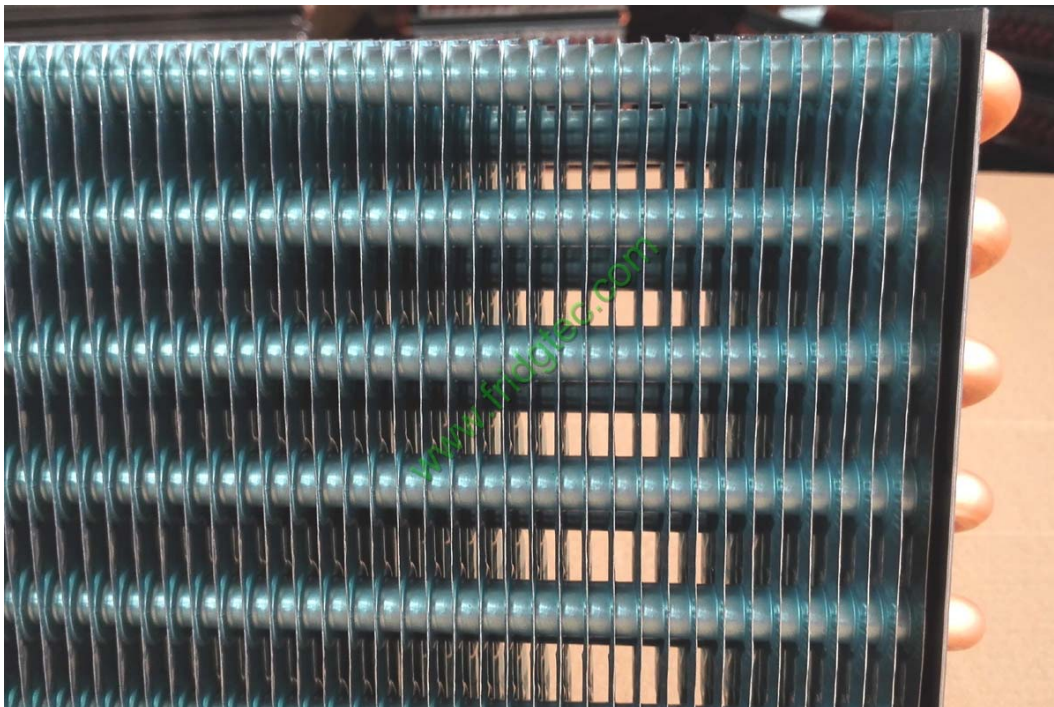
Aluminum fin drawing and expanding on copper tube, 100% wrapped the copper tube
