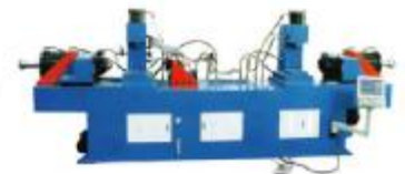
SG100NC-2H-3S Double head pipe end forming machine
