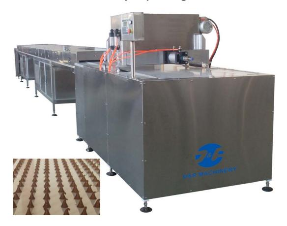
The machine is for depositing chocolate drops (chips). The chocolate drops/chips can be poured on the conveyor belt directly and the weight of the each drop can also be adjustable.
