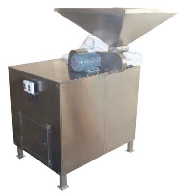
This machine is for grinding sugar to be sugar powder as required. The max. capacity is 250kg/hour.
