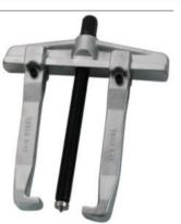
Heavy duty twin legged bar type puller, easy removal of pulleys, flywheels, bearings and gears, dropped forged chrome steel heat treated and chrome plated.thrust bearing prevents wear and damage to shaft.
