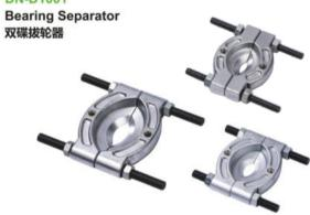
Designed for removing gears and bearings where access is available behind the item Two knife edges ensure a secure pulling surface Drop forged hardened alloy steel, used in conjunction with two leg mechanical pullers, hydraulic pullers or sliding beam
