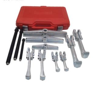
Heavy duty twin legged bar type puller, easy removal of pulleys flywheels, bearings and gears, dropped forged alloy steel, heat treated and chrome plated .thrust bearing prevents wear and damage to shaft.
