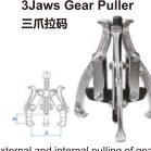
Puller with two reversible legs for external and internal pulling of gears, bearings, etc. Legs are forged carbon steel and have long and short reach facility. Yoke and thrust bolt are manufactured from carbon steel. Screw has a rolled thread with chemically blacked finish.
