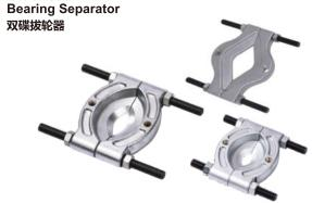
Designed for removing gears and bearings where access is available behind the item Two knife edges ensure a secure pulling surface Drop forged hardened alloy steel, used in conjunction with two leg mechanical pullers, hydraulic pullers or sliding beam
