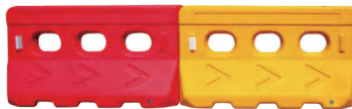
Name: Blowing Plastic barrier ATAR2203D Length: 1440mm Height: 780mm Width(Top/bottom): 140/310mm Water capacity: 250kg
