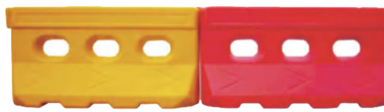
Name: Blowing Plastic barrier ATAR2203B Length: 1500mm Height: 800mm Width(Top/bottom): 250/480mm Water capacity: 250kg
