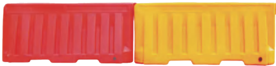
Name: Blowing Plastic barrier ATAR2208 Length: 2000mm Height: 800mm Width(Top/bottom): 200/400mm Water capacity: 400kg
