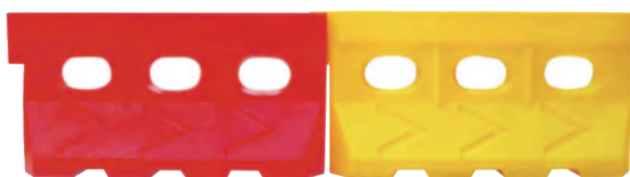
Name: Rotate moulding Plastic barrier ATAR2203A Length: 1500mm Height: 800mm Width(Top/bottom): 250/480mm Water capacity: 250kg
