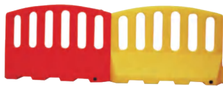
Name: Rotate moulding Plastic barrier ATAR2205A Length: 1500mm Height: 1200mm Width(Top/bottom): 150/430mm Water capacity: 200kg
