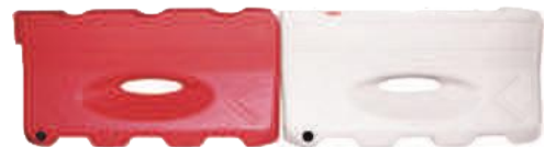
Name: Blowing Plastic barrier ATSM-1012 Length: 1300mm Height: 650mm Width(Top/bottom): 200/400mm Water capacity: 200kg
