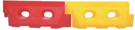
Name: Rotate moulding Plastic barrier ATSM-1007-1 Length: 1650mm Height: 650mm Width(Top/bottom): 150/400mm Water capacity: 250kg
