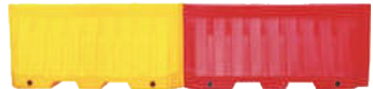
Name: Rotate moulding Plastic barrier ATSM-1008-1 Length: 2000mm Height: 800mm Width(Top/bottom): 145/400mm Water capacity: 400kg
