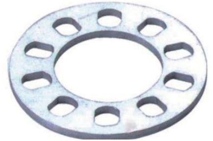
Part#: WS-102 Description: 5 Holes on 108-120mm Thickness:8mm I.D: 90mm O.D: 164.3mm
