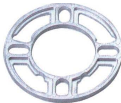
Part#: WS-109 Description: 4&5 Holes on 98-120mm Thickness:3mm,5mm,8mm I.D: 78.5mm O.D: 145mm
