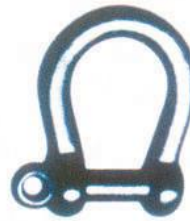
(3) SCREW PIN ANCHOR SHACKLE "BOW" TYPE WITHOUT COLLAR
