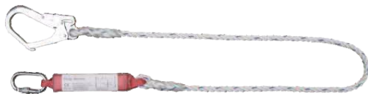
ATLS-9103 Safety Lanyard with Energy Absorber Material: 100% polyester Breaking Strength: 30KN Length: 1.8M-2M including the hook Rope Dia: 14mm With 1 alloy steel carabiner and 1 big forged snap hook Meet EN355 and EN354
