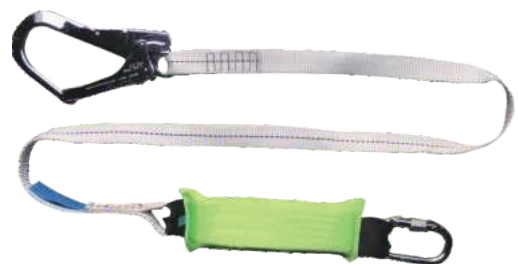
ATLS-9106 Safety Lanyard with Energy Absorber Material: 100% polyester Webbing width: 30mm Breaking Strength: 30KN Length: 1.8M-2M including the hook With 1 big alloy steel carabiner and 1 big forged hook Meet EN355 and EN354
