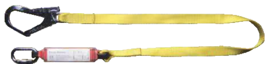
ATLS-9105 Safety Lanyard with Energy Absorber Material: 100% polyester Webbing width: 30mm Breaking Strength: 30KN Length: 1.8M-2M including the hook With 1 big alloy steel carabiner and 1 big forged hook Meet EN355 and EN354
