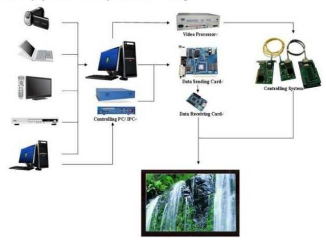
Module-Cabinet-LED display screen configuration diagram
