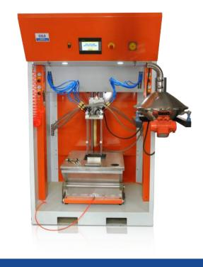
The key to a quick and clean color change is the compact powder center. exhaust air system, it offers maximum user comfort! can be upgraded with a fresh powder supply and a disposal system for used powders. .
