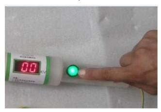
3. Press the gun trigger and let the gun electrode touch the metal ball then can read the output of voltage.
