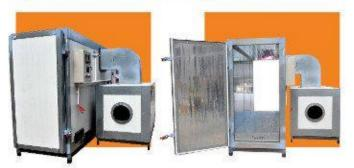
Industrial curing batch oven, front and back door,heat Source:LPG
