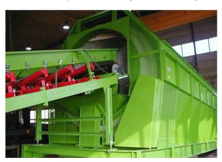
design dimensions of the diameter of aperture of the sieving disk respectively manufacture, we could replace the sieving disk timely, resolves the malpractice that the sieving disk can not be replaced. The sieving effect much better than the traditional
