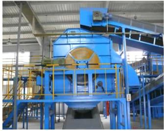
independently produced by our company, in the process of sorting and separating and disposal the urban residential house refuse, the use effect is extremely well, the bag-breaking rate achieves above 90%.
