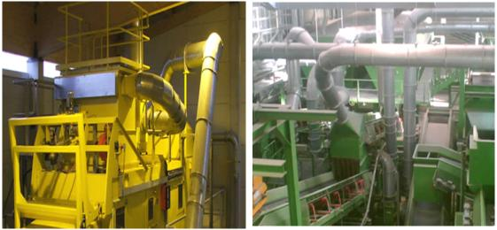
to achieve the purpose of sorting  $\$  recovering and recycling the garbage. The air classification equipment independently developed and manufactured by our company have the features that the power is low, noise is small and the air classification effect is well. There are two kinds of this production. One is positive pressure fanning machine; the other is negative pressure fanning machine.
