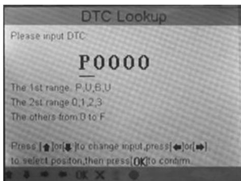
You can use [**▲**] [**▼**] key to change the first letter. It can be switched among "P", "B", "C" and "U". And press [**OK**] moves the cursor to next. And then press [**▶**] [**◀**] key to input number. After you input the code number, press [**OK**] to view the definition of the code.
