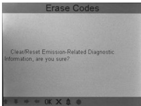
Press [ **OK** ] to erase DTC's, and the screen will display the interface as shown below:
