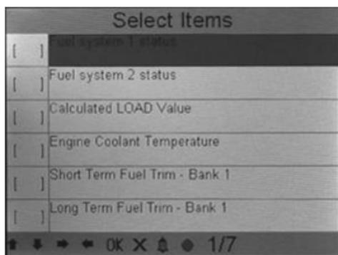
You can use [▶] [◀] button to turn page, and press [▲] [▼] button to select data stream items, then press [**OK**] button to confirm the selected items, the screen will display the interface as shown on the next page:
