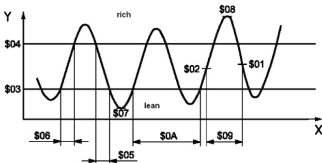
Select [**O2 Sensor Monitor Test**] in the [Diagnostic Menu] and press [**OK**] and the screen will display as shown below:
