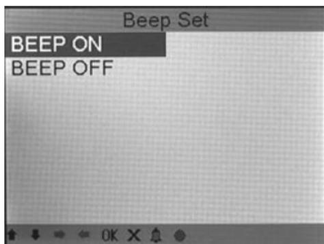
Press [**OK**] to select ON/OFF. When this function is ON, the icon “
