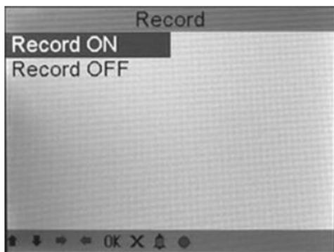
Press **[OK]** to select ON/OFF. When this function is ON, and the icon “
