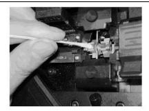
3. If fibers are still not in the right place, enter "Manual mode" and press ▲ or ▼ to align them, then set to "auto mode" again. Make sure the movement of fiber and key-press is in the same direction.
