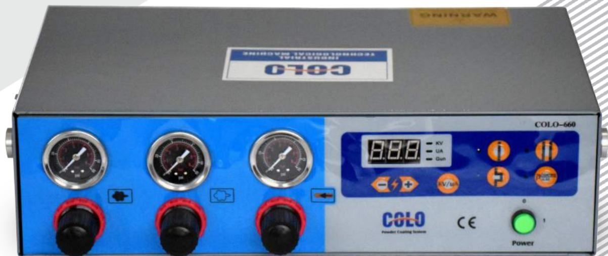
Control unit has one-touch intelligent operation button good for flat parts, complicated parts, recoat parts and impulse function. Easy to operate.
