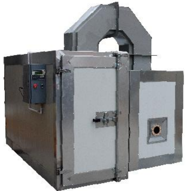
Industrial curing batch oven. front and back door, heat Source: LPG
